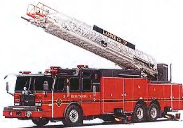
**Aerial Platform:** heavy duty tandem axle fire truck equipped with a very large ladder, also includes a secured bucket (platform) at the tip of the ladder, hydraulically operated that extends from the truck and cannot be removed from the truck, most commonly equipped with a 75 – 100-foot ladder.
