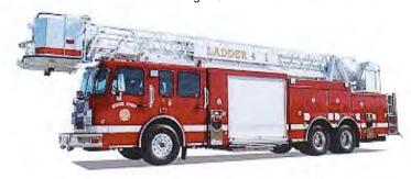
**Ascendant Aerial Platform**: single axle fire truck equipped with a very large ladder, also includes a secured bucket (platform) at the tip of the ladder, hydraulically operated that extends from the truck and cannot be removed from the truck, most commonly equipped with a 107 – 110-foot ladder.
