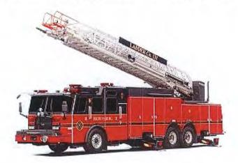
**Aerial Platform:** heavy duty tandem axle fire truck equipped with a very large ladder, also includes a secured bucket (platform) at the tip of the ladder, hydraulically operated that extends from the truck and cannot be removed from the truck, most commonly equipped with a 75 – 100-foot ladder.
