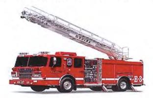
**Aerial:** heavy duty tandem axle fire truck equipped with a very large ladder, hydraulically operated that extends from the truck and cannot be removed from the truck, most commonly equipped with a 75 – 100-foot ladder.
